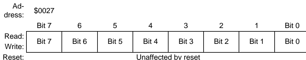
Figure 8-21. Pulse Accumulator Count Register (PACNT)
