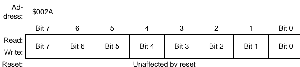
Figure 7-5. SPI Data I/O Register (SPDR)
